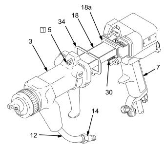
1 Tighten to 18 in-lbs (2 N•m) **maximum** (about half turn past snug), using wrench provided.
